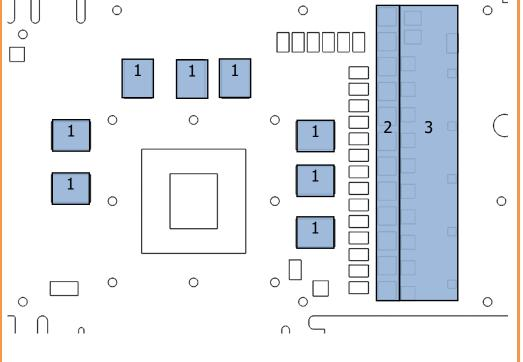
3. CUTTING THERMAL PADS: Your block comes with thermal pads, some of which are already pre-cut. Others have to be cut to smaller chunks in order to cover all the VRM components such as MOSFETs and drivers. PLEASE REMOVE THE PROTECTIVE FOIL FROM BOTH SIDES OF THE THERMAL PADS PRIOR TO INSTALLATION.
